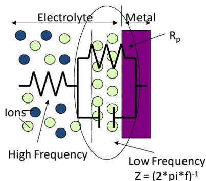
This situation is exploited by ac methods. The instrumentation for ac methods is more complex, the mathematics are more sophisticated, extensive modeling is required, and it takes experience to identify the correct model. Nonetheless, ac methods can provide superior, often unique, insight about the corrosion rate and mechanism.
