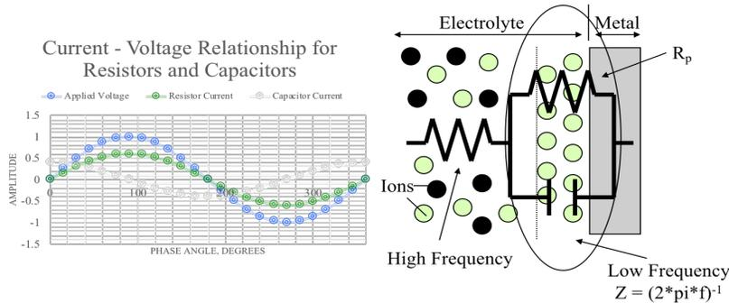
The rate of chemical processes sets limits on the frequency that each process can follow, so the voltage-current data is collected over a wide range of frequencies, allowing the various processes to be measured independently. The voltage-current data is modeled as an electrical circuit of resistors, capacitors, and other elements, which is fit to the data using non-linear least squares. Each element of the circuit models a particular chemical process as shown above.
